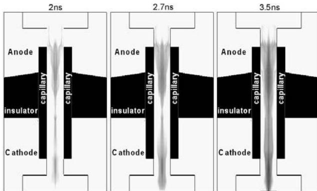
**Figure 2:** Preionization dynamics of a capillary discharge with iso-contours of ion density  $n_i$  shown at different times.
