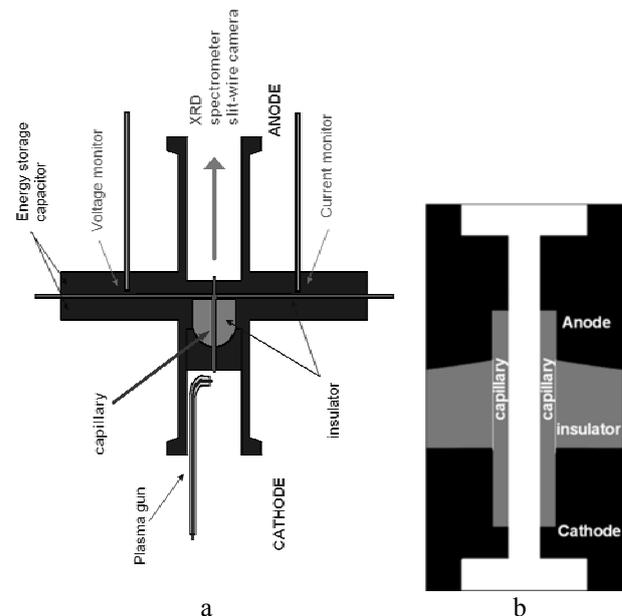
**Figure 1:** a) Geometry of the EPPRA MPP capillary discharge; b) – zoomed view of the capillary region adopted for simulation.
