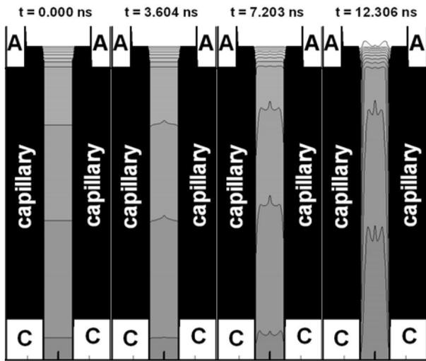
**Figure 3:** Capillary discharge dynamics in argon with a pressure gradient filled capillary; iso-density contours shown at different time moments.
