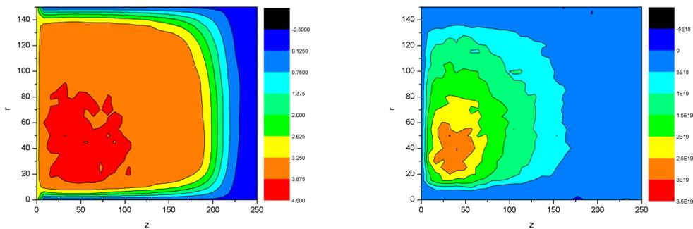
Fig. 1 - Plasma potential (V) and electron density (m<sup>-3</sup>) inside the acceleration channel.
