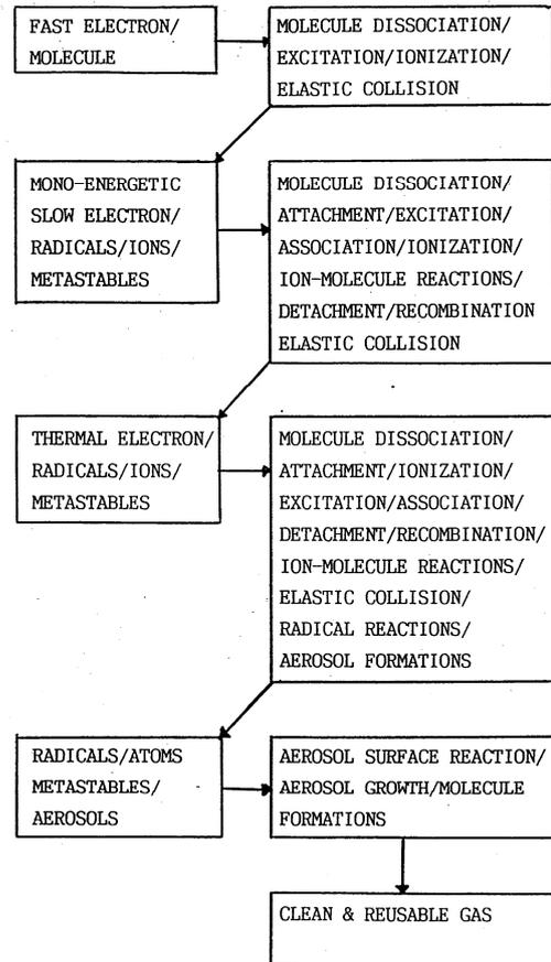
Fig.1 Mechanism of plasma pollution control [1].
