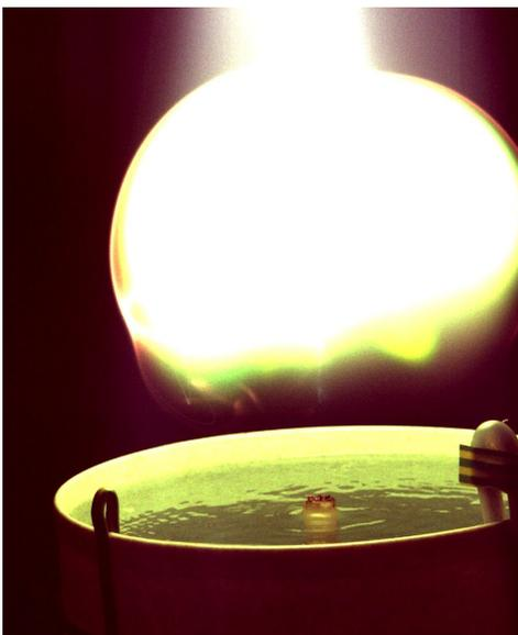
**Fig .3:** Plasmoid 30 ms after current zero. The diameter is about 0.2 m.
