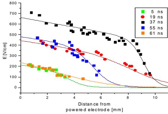
Fig. 5: Space and phase resolved electric fields in a strongly asymmetric CCRF discharge (Kr, 1 Pa, 8 W)
