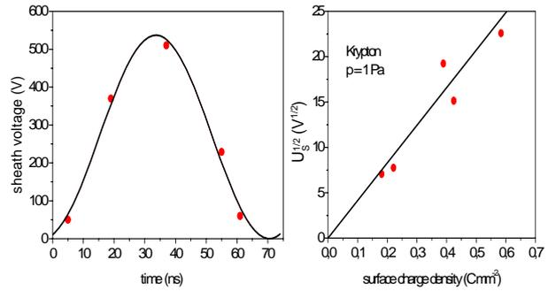
Fig. 7: Comparison between measured (high-voltage probe) and calculated sheath voltages (E-fields) and sheath voltage vs. surface charge density
