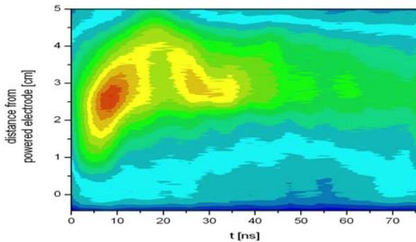
Fig. 10: Space and phase resolved excitation into Ne2p<sub>1</sub> in a neon discharge at 2 Pa and 8 W
