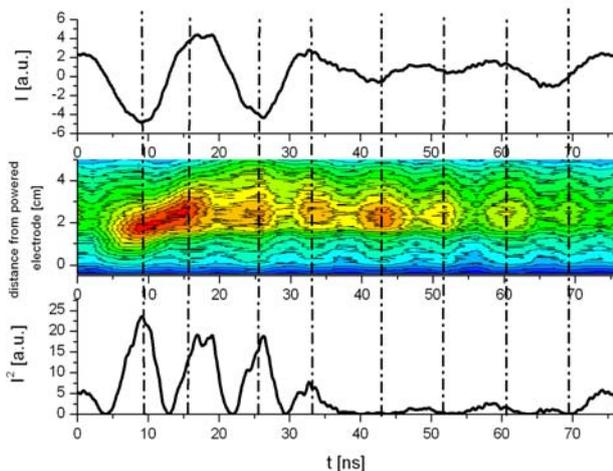
Fig. 11: Space and phase resolved excitation into Kr2p<sub>5</sub> and current in a krypton discharge at 0.5 Pa and 8 W
