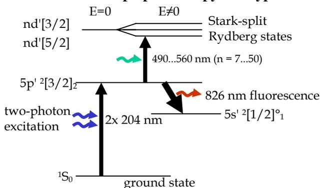
Fig. 3: Excitation scheme in krypton used for FDS
