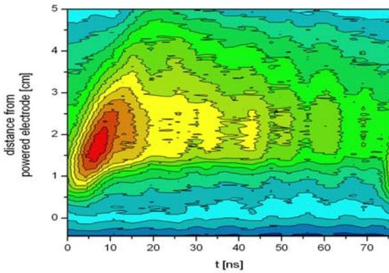
Fig. 6: Space and phase resolved excitation into Kr<sub>2p<sub>5</sub></sub> in a krypton discharge at 1 Pa and 8 W (gatewidth 4.2 ns)
