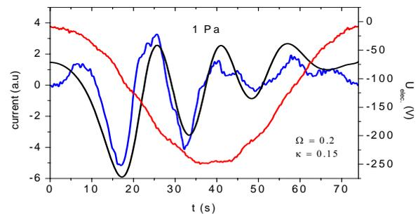
Fig. 12: Measured (blue) and modelled (black) current to the chamber wall and RF-voltage in Kr at 1 Pa and 8 W.
