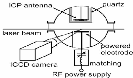
Fig. 2: GEC reference cell accessible for FDS and PROES
