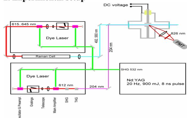
Fig. 1: Laser system and calibration cell
