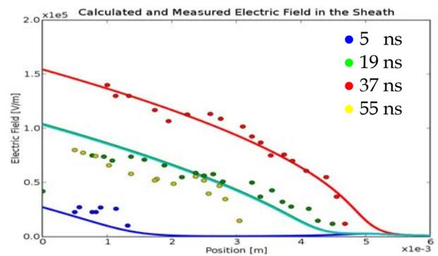
Fig. 9: Comparison between measured (points) and calculated (lines) electric fields (Kr, 10 Pa, 8 W)
