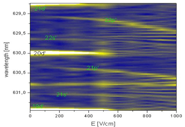
Fig. 4: Measured Stark map in krypton in the range 19d'-21d'. The fluorescence decrease is indicated by bright lines
