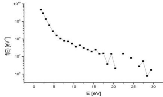
Fig. 8: EEDF obtained from langmuir probe measurements 2,5 cm above the powered electrode in pure Kr at 10 Pa and 8 W
