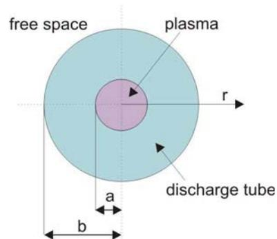
Fig. 1. Cross section of wave-guiding structure.
