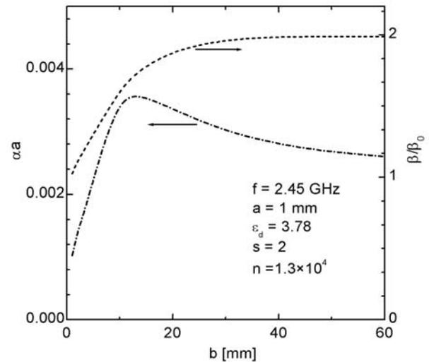
Fig. 3. The normalized attenuation  $\alpha a$  and normalized phase  $\beta/\beta_0$  coefficients vs. the discharge tube outer radius  $b$ , for constant values of  $n$  and  $s$ .
