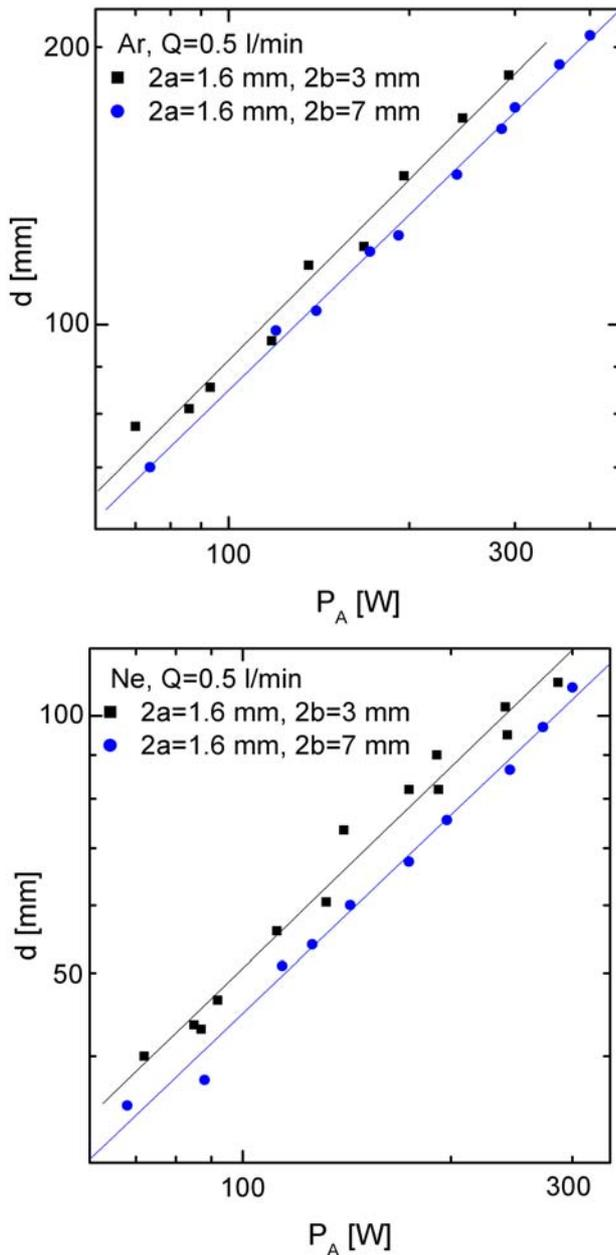
Fig.6. The dependence of the average plasma column length on absorbed microwave power for discharge in (a) argon and (b) neon. The experimental results (points) are approximated by straight lines.
