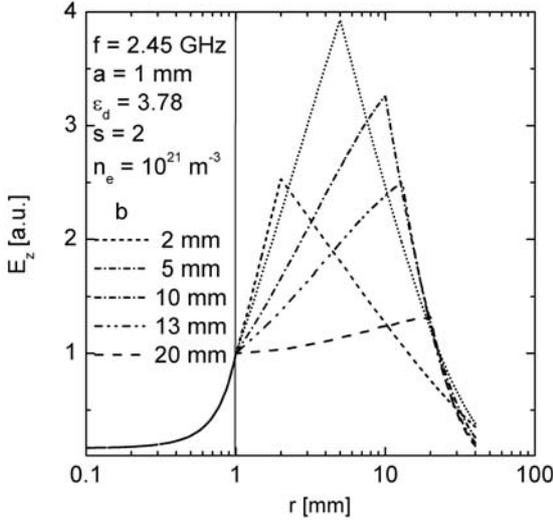
Fig. 4. Radial distribution of the axial component of the electric field  $E_z$  for different values of  $b$ .
