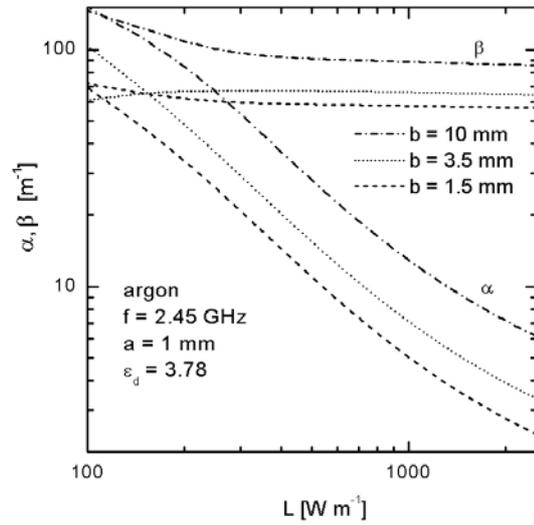
Fig. 5. Attenuation  $\alpha$  and phase  $b$  coefficients as functions of  $L$  for various values of  $b$ .
