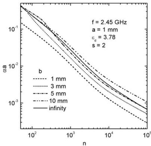
Fig. 2. Normalized attenuation  $\alpha a$  vs. the normalized electron concentration  $n$ , for various values of the discharge tube outer radius  $b$ .
