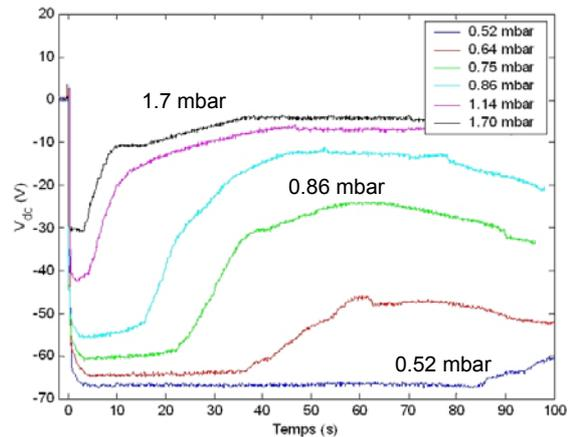
Fig.6. Dust formation as function of pressure
