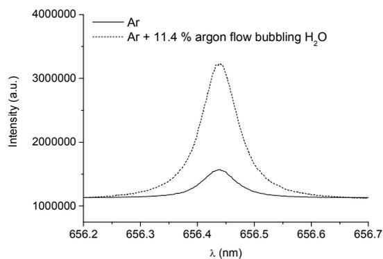
Figure 3.  $H_\alpha$  line intensity in an argon and an argon-water plasma column.
