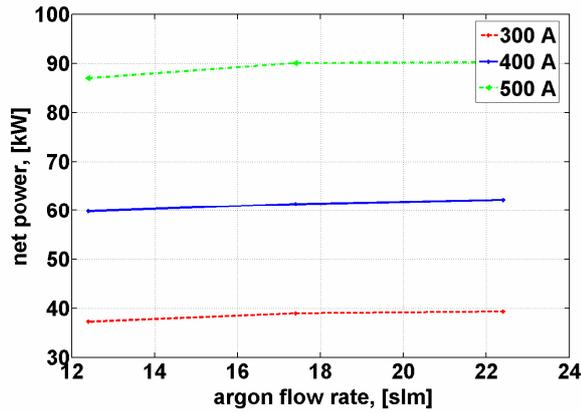
Figure 4: Net power of the torch as a function of the argon flow rate for different arc currents.
