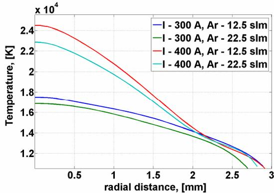
Figure 5: Temperature profiles, measured at the torch exit nozzle for different operation conditions.
