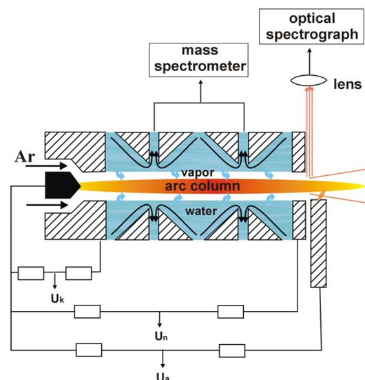
Figure 1: The plasma torch with the gas-water stabilisation of the arc and applied diagnostics.
