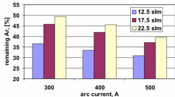
Figure 6: Argon remaining in the plasma after leaving the plasma arc chamber for different conditions.
