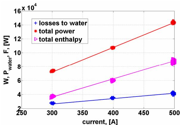
Figure 2: Power balance in the torch as a function of the arc current for Ar – 12.5 slm.
