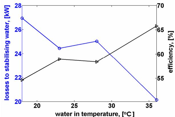
Figure 3: Dependence of the arc characteristics on the temperature of the stabilizing water.
