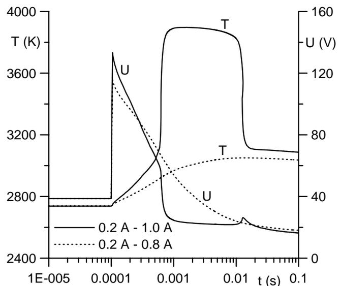
Figure 2: Modelling results for the maximum cathode temperature (T) and near-cathode voltage drop (U) for different current jumps imposed to a cathode operating in the mercury plasma.
