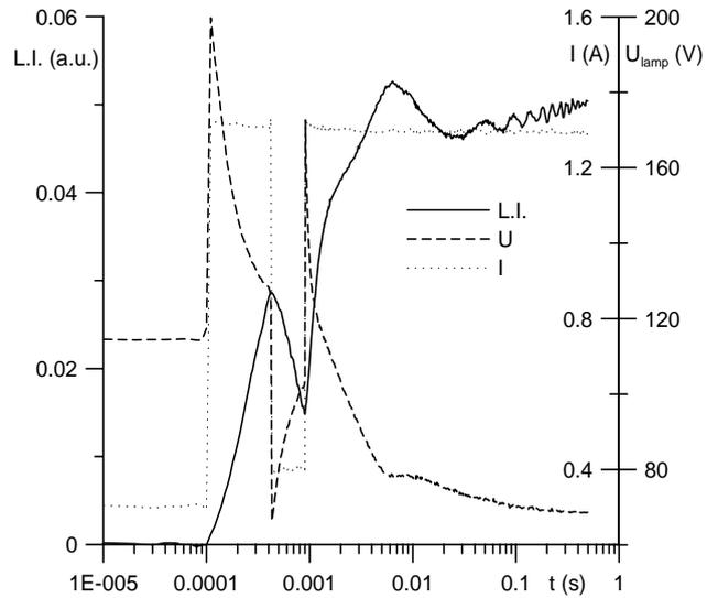
Figure 6: experiments: the prevention of a diffuse-spot-diffuse transition in a  $0.2\text{ A} - 1.0\text{ A}$  current jump.  $U$ : lamp voltage;  $I$ : lamp current.
