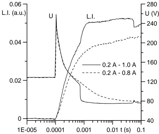
Figure 3: Experimental results for the lamp voltage,  $U$ , light intensity in the near-cathode region, L.I., for different current jumps imposed to a type 1 typical lamp.
