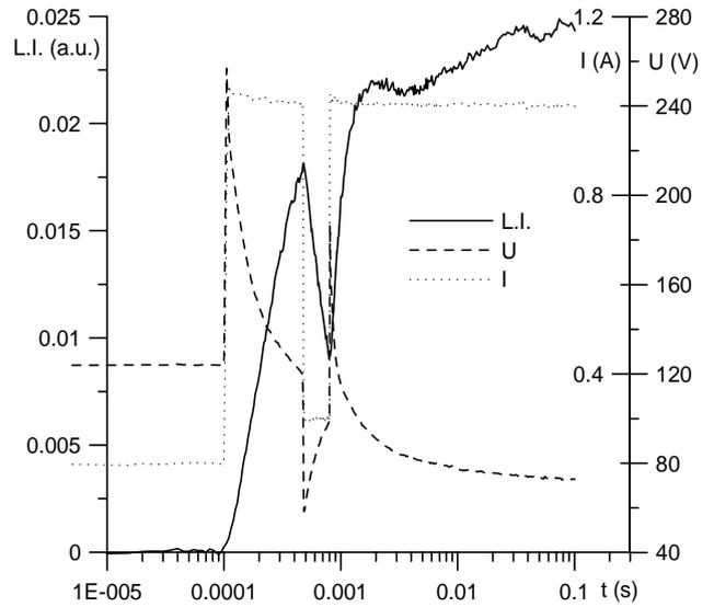
Figure 5: experiments: the prevention of a diffuse-spot-diffuse transition in a  $0.2\text{ A} - 1.0\text{ A}$  current jump.  $U$ : lamp voltage;  $I$ : lamp current.
