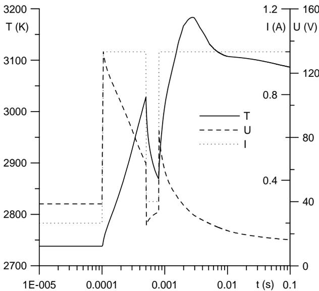
Figure 4: modelling: the prevention of a diffuse-spot-diffuse transition in a  $0.2\text{ A} - 1.0\text{ A}$  current jump.  $T$ : maximum cathode temperature  $U$ : near-cathode voltage drop;  $I$ : current.
