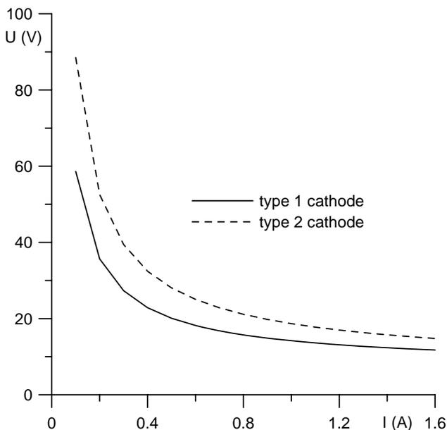
Figure 1: CVC of the near-cathode plasma layer for type 1 and average type 2 cathodes (modelling).
