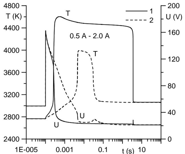
Figure 4. Maximum temperature on the cathode surface and near-cathode voltage drop for a current jump. 1: cathode in the form of a rod with a flat front surface. 2: cathode in the form of a rod with a rounding edge at the front surface.
