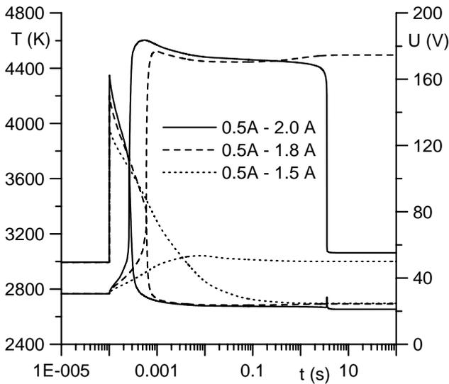
Figure 3. Maximum temperature on the cathode surface and near-cathode voltage drop for different current jumps. Cathode in the form of a rod with a flat front surface.
