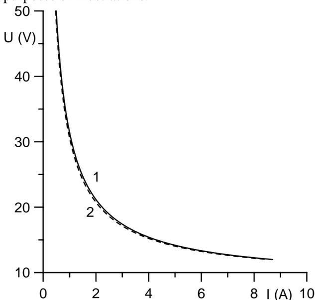
Figure 1. Current-voltage characteristics of the diffuse mode. 1: thermal conductivity of tungsten taken from [8]. 2: thermal conductivity of tungsten taken from [11].
