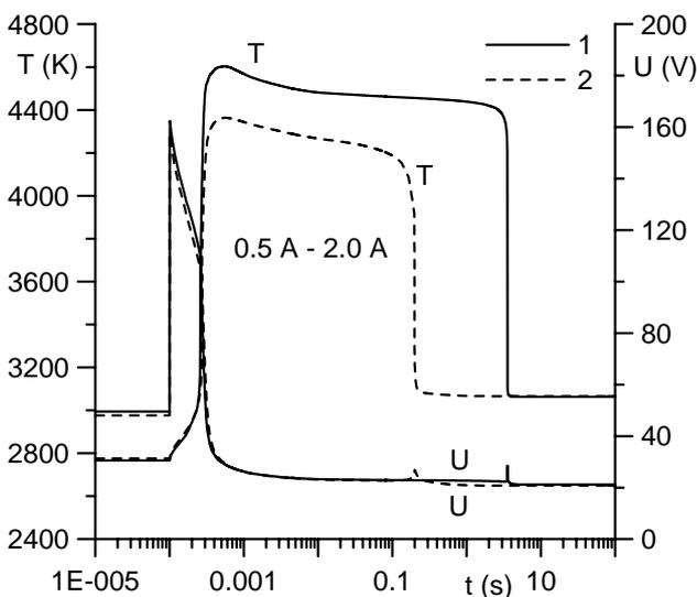
Figure 5. Maximum temperature on the cathode surface and near-cathode voltage drop for a current jump on a cathodes in the form of a rod with a flat front surface. 1: thermal conductivity of tungsten taken from [9]. 2: thermal conductivity of tungsten taken from [2].
