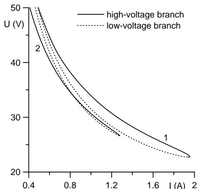
Figure 2. Current-voltage characteristics of the spot mode. 1: thermal conductivity of tungsten taken from [8]. 2: thermal conductivity of tungsten taken from [11].
