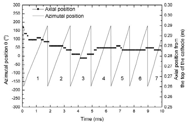
Figure 6 : Evolution of the arc root position versus time.
