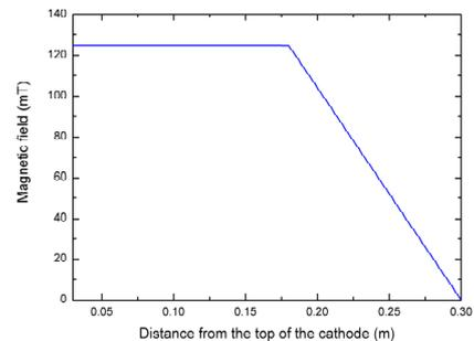
Figure 3 : Magnitude of the magnetic field in the cathode
