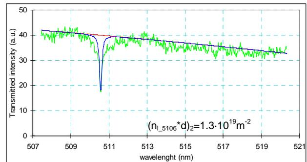
Figure 3. Arc spectre and its best fit (new electrodes)
