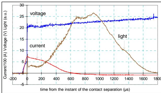
Figure 2. Evolutions of arc voltage, current and light
