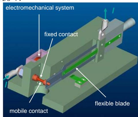
Figure 1. Experimental sketch of the circuit breaker
