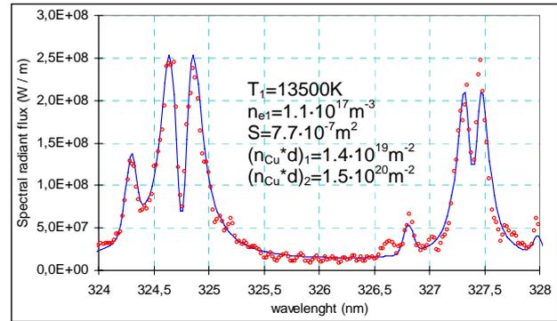
Figure 4. Arc spectre and its best fit (resonance lines)
