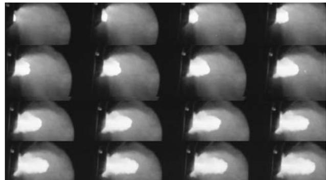
Fig. 5. Development of hydrogen-enriched plasma jet:  $U_0 = 900 \text{ V}$ ,  $Q = 100 \text{ J}$ . Shooting time is 8 μs
