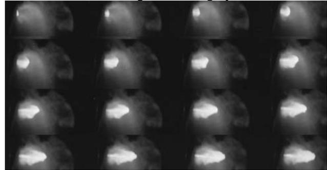
Fig. 4. Development of hydrogen-enriched plasma jet:  $U_0 = 16 \text{ kV}$ ,  $Q = 100 \text{ J}$ . Shooting time is 8 μs
