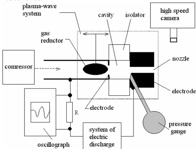
Fig. 3 Schematic of the experimental set-up
