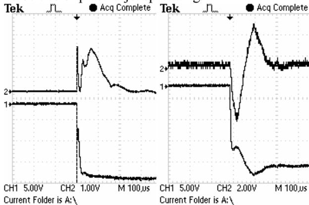
Fig. 2 Typical voltage (1) and current (2) oscillograms of driven arc (on the left) and the oscillograms in the case of the shot circuit (on the right)
