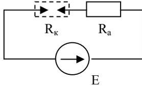
Fig. 1 Electric discharge circuit:  $R_k$  is the ohmic resistance of the discharge gap,  $R_a$  is the external ohmic resistance,  $E$  is the source of electromotive force
