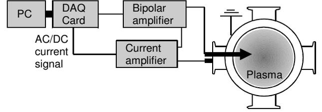
Fig. 3. Setup of the Boyd-Twiddy probe system.
