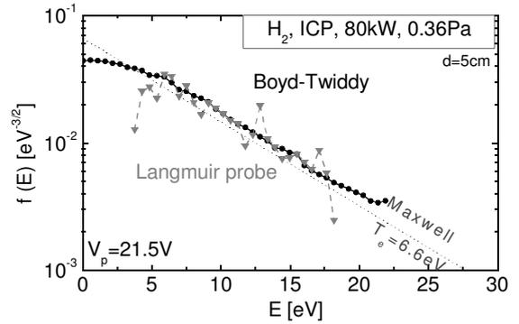
Fig. 6. EEDFs in an ICP hydrogen plasma.
