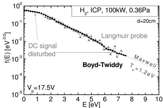
Fig. 5. EEDFs in an ICP hydrogen plasma.
