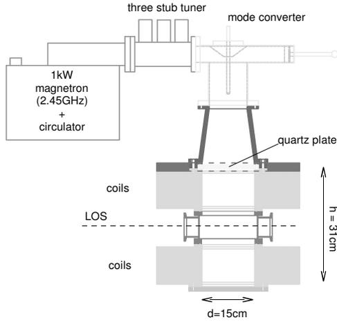
Fig. 2. Setup of the ECR plasma.
