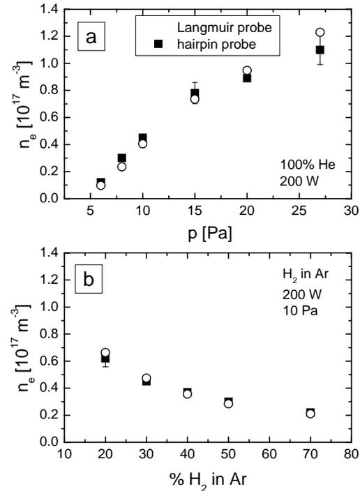
Figure 1: Comparison of the hairpin resonance probe with the Langmuir probe in Helium (a) and Argon plasmas with hydrogen admixture (b)
