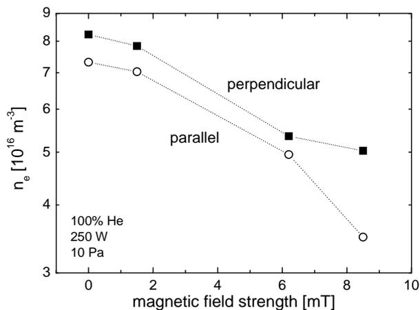
Figure 3: Electron densities in helium plasmas with increasing magnetic field strength, probe tip parallel and perpendicular to the field lines
