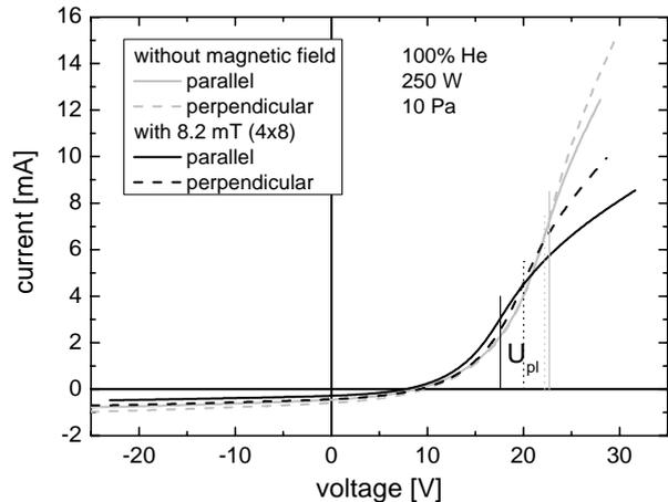
Figure 2: Voltage/current characteristics of Langmuir probe measurements with and without magnetic field in helium plasmas
