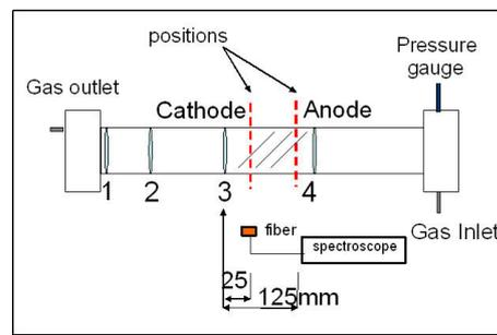
Figure.1 Schematic of experimental apparatus.
