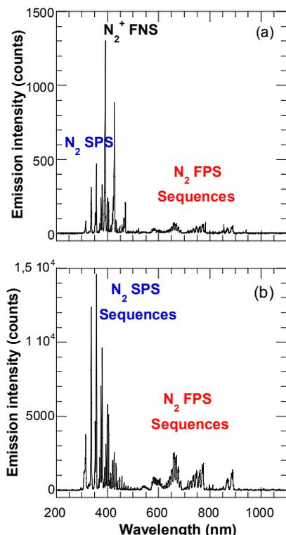
Figures 2a-b. OES spectra of  $N_2$  dc discharges very close to (a) the cathode, 3mm, and (b) the anode, 1mm, obtained at 3 Torr and 50 mA.
