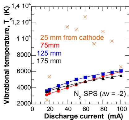
Figure 4. Vibrational temperatures as a function of discharge current at the four axial positions far from the cathode.
