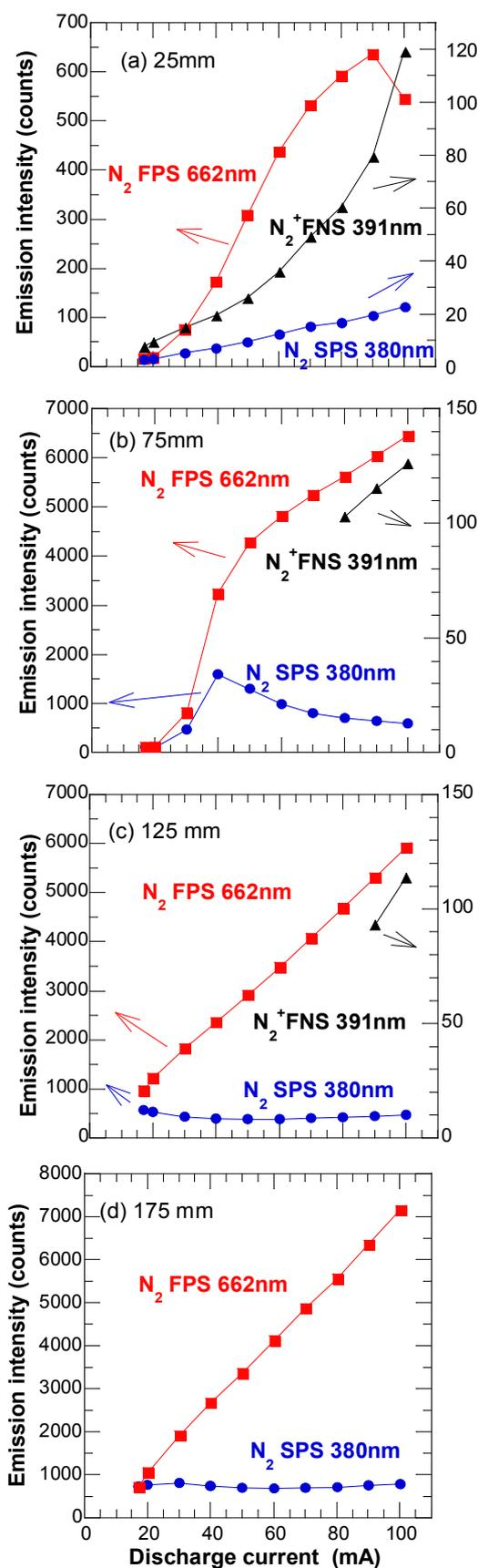
Figures 3a-d Emission intensities of SPS (380.4 nm), FPS (662.4 nm) of  $N_2$  molecule, FNS (391.4 nm) of  $N_2^+$  molecular ion vs discharge current at (a) 25 mm, (b) 75 mm, (c) 125 mm and (d) 175 mm far from the cathode.
