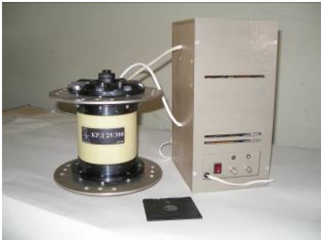
Fig.3. RSD-switch (switch type KRD-25-300) for operating current of up to 300 kA and operating voltage of up to 25 kV (left) with trigger generator (right) connected in parallel.
