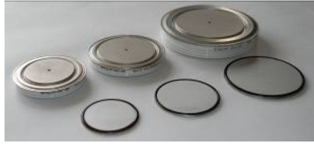
Fig.2. Reverse – switched dinistors for peak current from 200 kA to 500 kA and blocking voltage of 2400 V, encapsullated in hermetic metal – ceramic housing and without housing (RSD sizes of 64, 76, and 100 mm)
