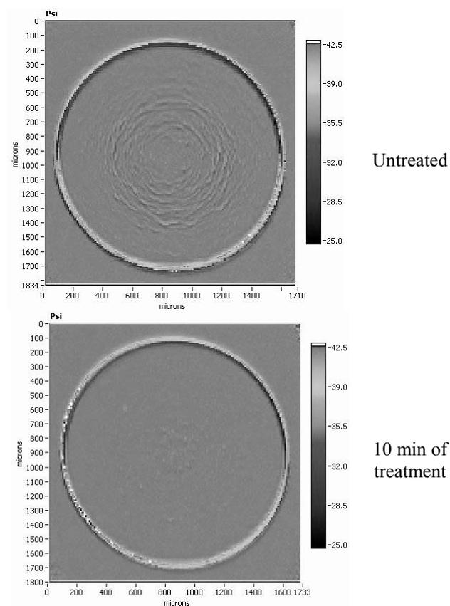
Fig. 4. Ellipsometric image of BSA before and after plasma treatment in  $O_2/H_2$  50:50 discharge.
