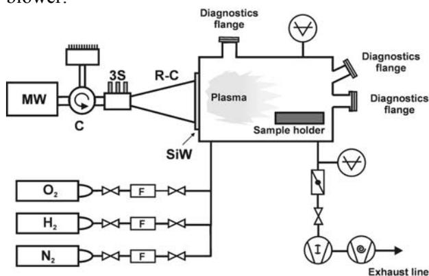
Figure 1. Schematics of plasma reactor
