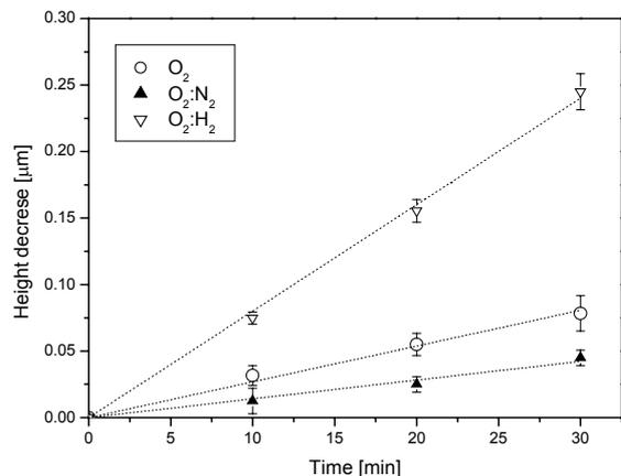
Fig. 5. Decrease of the BSA thickness after a plasma treatment (16 Pa, 100 sccm, and applied MW power 1000W)
