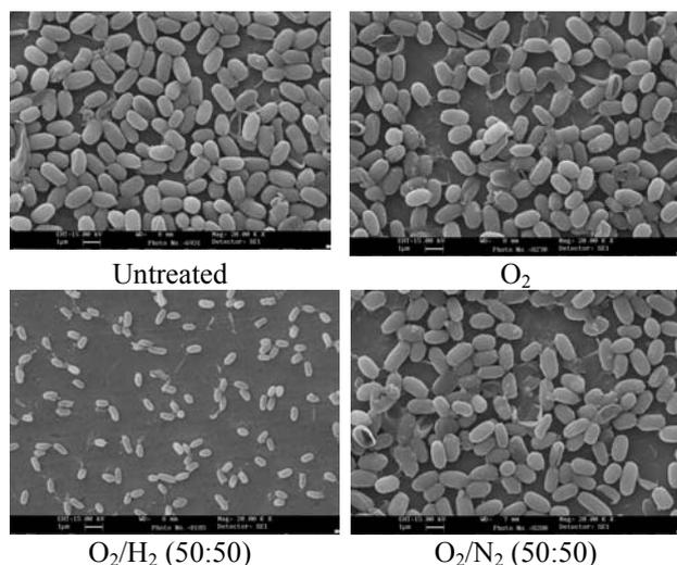
Fig 2. Scanning electron microscope images of untreated and plasma treated bacterial spores (Applied MW power 1000 W, treatment time 1 min, pressure 16 Pa, total gas flow 100 sccm).
