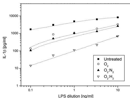
Fig. 3. Comparison of the plasma treatment efficiency LPS in different discharges measured by the human whole blood incubation and following IL-1 $\beta$  ELISA. (Applied MW power 1000W, treatment time 1 min, pressure 16 Pa, total gas flow 100 sccm).
