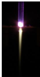
Fig. 3. Photograph of the generated micro-plasma torch (nozzle i.d.: 0.6 mm)
