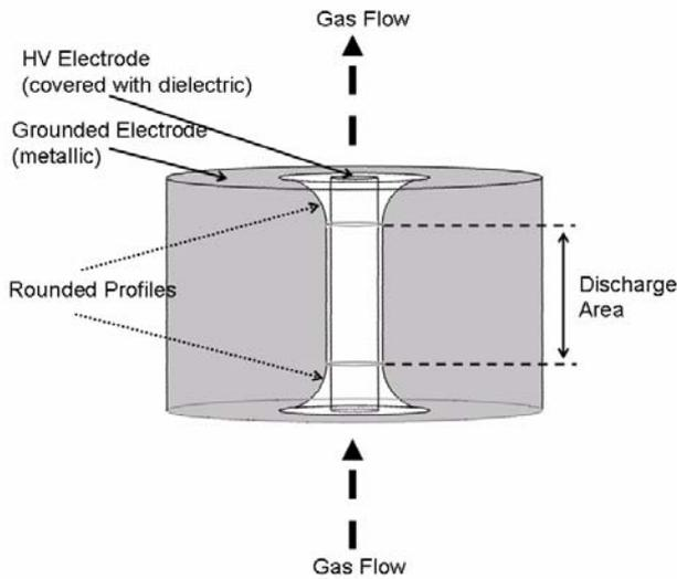
**Figure 1:** Sketch of the DBD reactor
