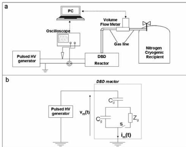
**Figure 4:** (a) Schematic representation of the experimental set-up (b) Electrical equivalent
