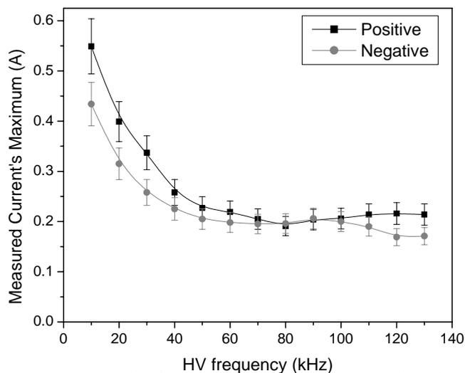
**Figure 6:** Absolute measured current's maxima for the negative and positive HV pulse.
