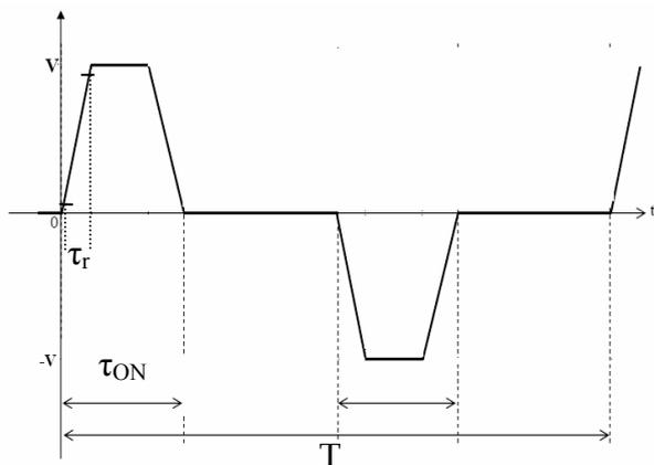
**Figure 2:** Idealized HV generator output signal
