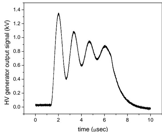
**Figure 3:** Positive voltage pulse at the generator's output (no load)
