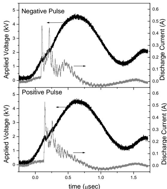
**Figure 6:** Measured voltage and current waveforms for the negative and positive HV pulse. (Negative signals have been inverted).
