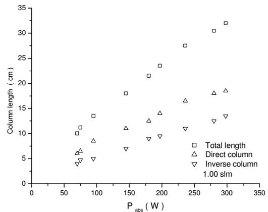
Fig. 4 Lengths of direct and inverse columns, flow 1.00 slm
