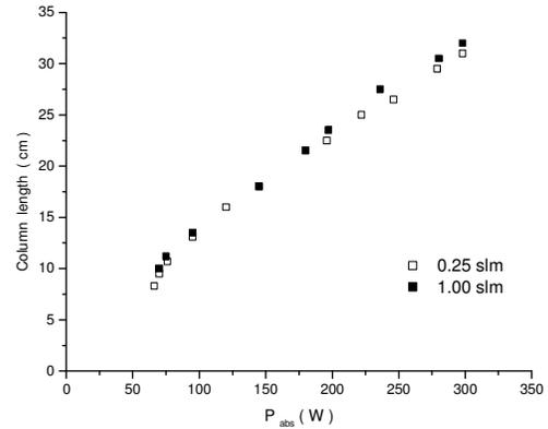
Fig.2 Column length as function of the absorbed power
