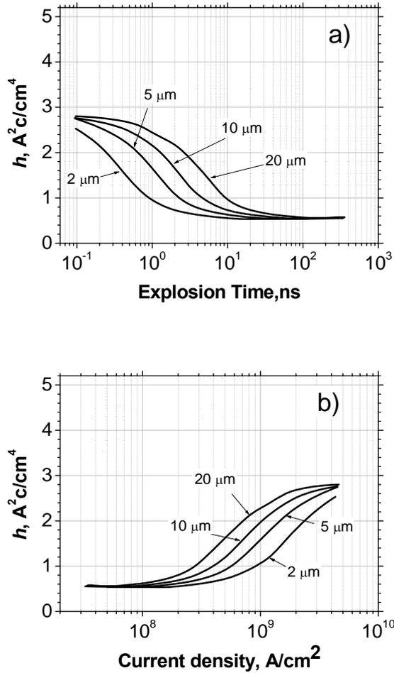
Fig. 1. Specific action integrals versus explosion time (a) and current density (b) for the explosion of wires of diameter 2, 5, 10, and 20 μm.
