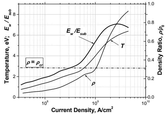
Fig. 2. Thermodynamic parameters of the metal of a wire versus current density at the explosion time,  $\tau_{ex}$ .
