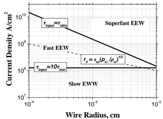
Fig. 3. Diagram of EEW modes for aluminum conductors.
