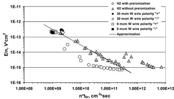
Fig. 6. Dependence of the parameter  $E_{br}/n$  on  $n \cdot \tau_{br}$  observed in experiments on the breakdown of a gap filled with hydrogen with and without UV preionization and in experiments on the electric explosion of a 6.35- $\mu\text{m}$  and 30.48- $\mu\text{m}$  tungsten wire in
