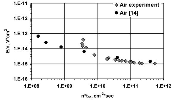
Fig.5. Dependence of the parameter  $E_{br}/n$  on  $n \cdot \tau_{br}$  observed in experiments on the breakdown of the gap filled with air.
