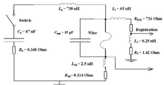
Fig. 1. Electric circuit of the RLC generator.
