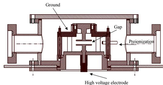
Fig. 3. Schematic of the vacuum chamber with the gas-filled gap load.
