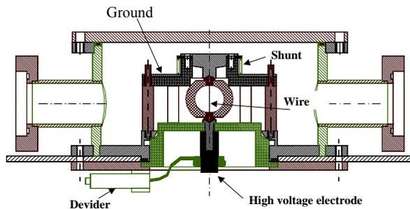
Fig. 2. Schematic of the vacuum chamber with the fine wire load.
