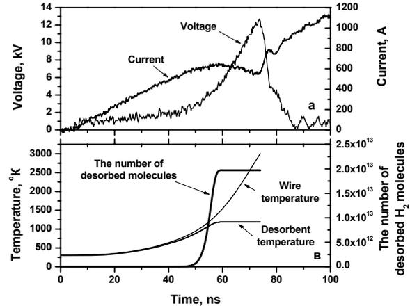
Fig.4 a- current and voltage oscillograms, b – estimation of the wire temperature, desorbed gas temperature and number of desorbed  $H$  atoms.
